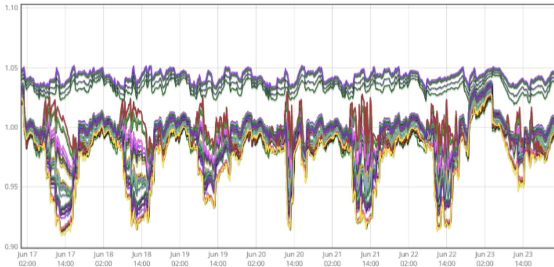
**Figure 49 – Low-Voltage OLTC Case – Grid Situation (one summer week in June)**
