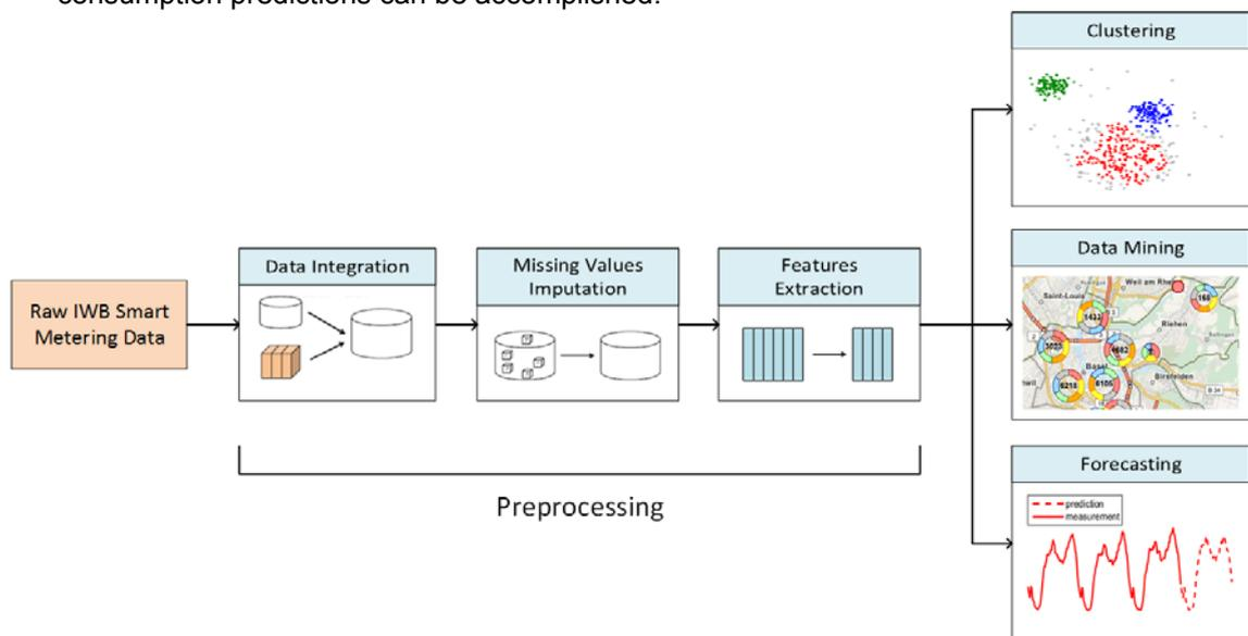
Figure 27 – Smart Meter Data Analytics Approach
