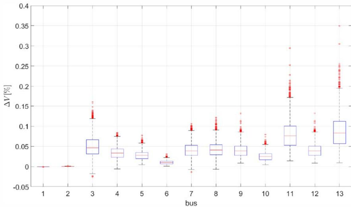
**Figure 15** – IWB *Kleinhünigeranlage*: instantaneous voltage error per bus for  $\{P, Q, V\}$  measurements at 2 buses
