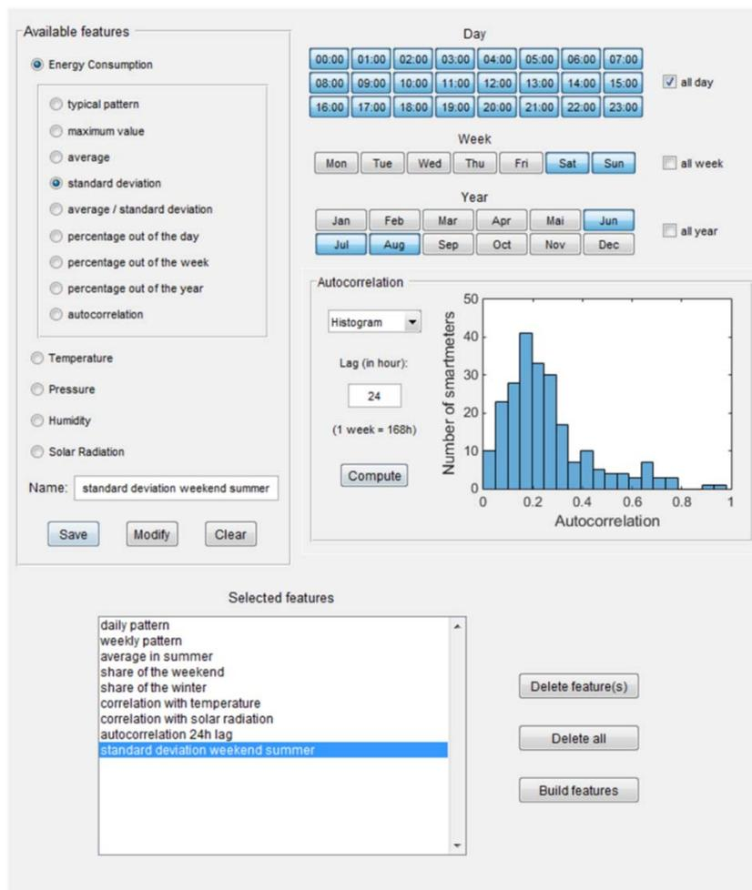
Figure 29 – Graphical User Interface for Features Selection
