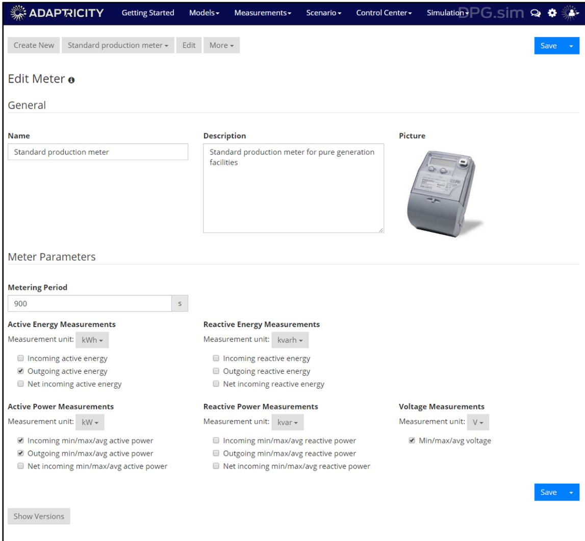
Figure 4 – Screenshot of Smart Metering parameterization interface in DPG.sim
