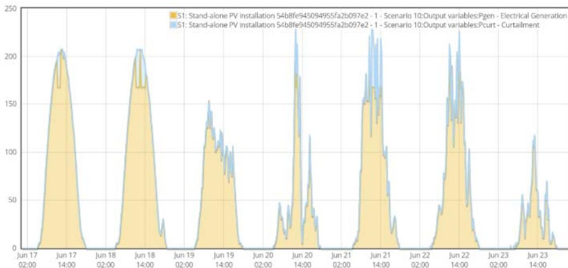
Figure 45 – PV Curtailment Case – Grid Situation (one summer week in June)
