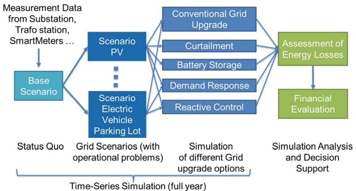
Figure 41 – Smart Grid Upgrade Option Evaluation Methodology
