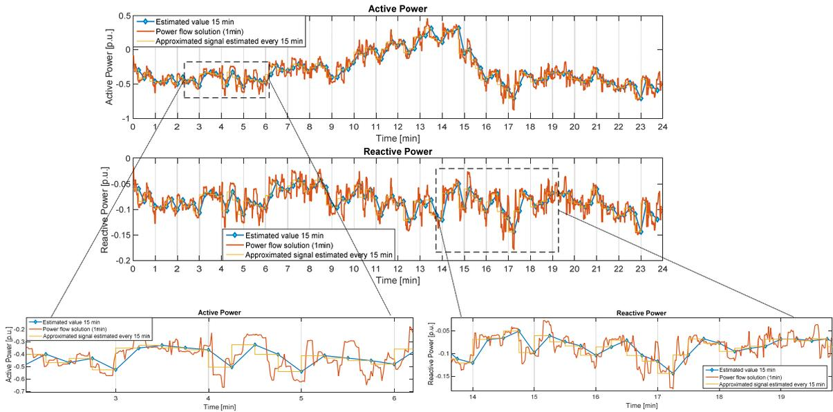
**Figure 13 – Active and Reactive power at bus 3.**
