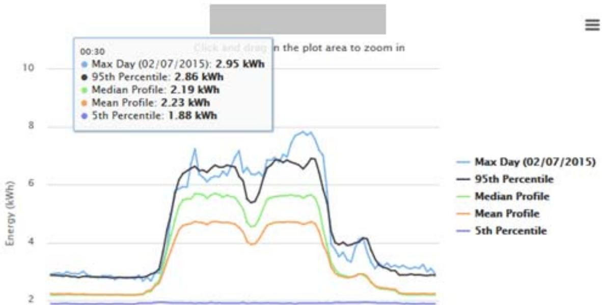
Figure 34 – Typical Daily Pattern of a Specific Industrial Customer
