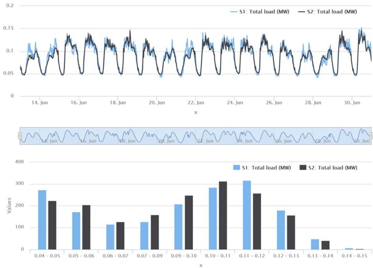
**Figure 23 – Active Power Flows at a Transformer & Histogram with Measured (blue) and Predicted (black) Data**
