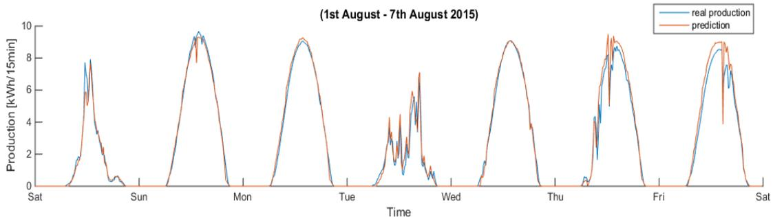
Figure 40 – Day-Ahead Production Forecast for a PV System
