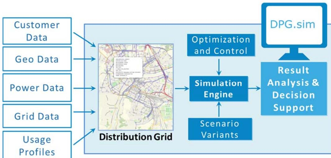
Figure 3 – Structure of Simulation Platform *DPG.sim*.
